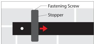
**Step 5:** Take the 10mm Wall anchor. Remove the Spacers from the pre assembled Wall Anchor and slide the 10mm wall anchor through the per-drilled holes on the rail. Now slide the spacer back onto the wall anchor and place the wall anchor into the drilled hole in the wall. With a hammer, gently nail the wall anchor into the wall, making sure not to bend the wall anchor.
