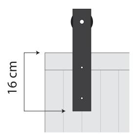
**Step 6:** Mounting the Hanging systems to the door. Make sure to measure the hanging brackets precisely 16cm from the top of the door.
